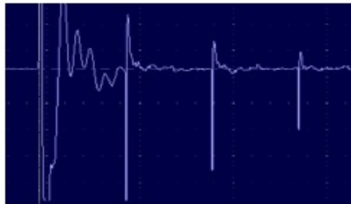
Figure 8 : Laser ultrasonic signal obtained with a 5mm-thick steel
